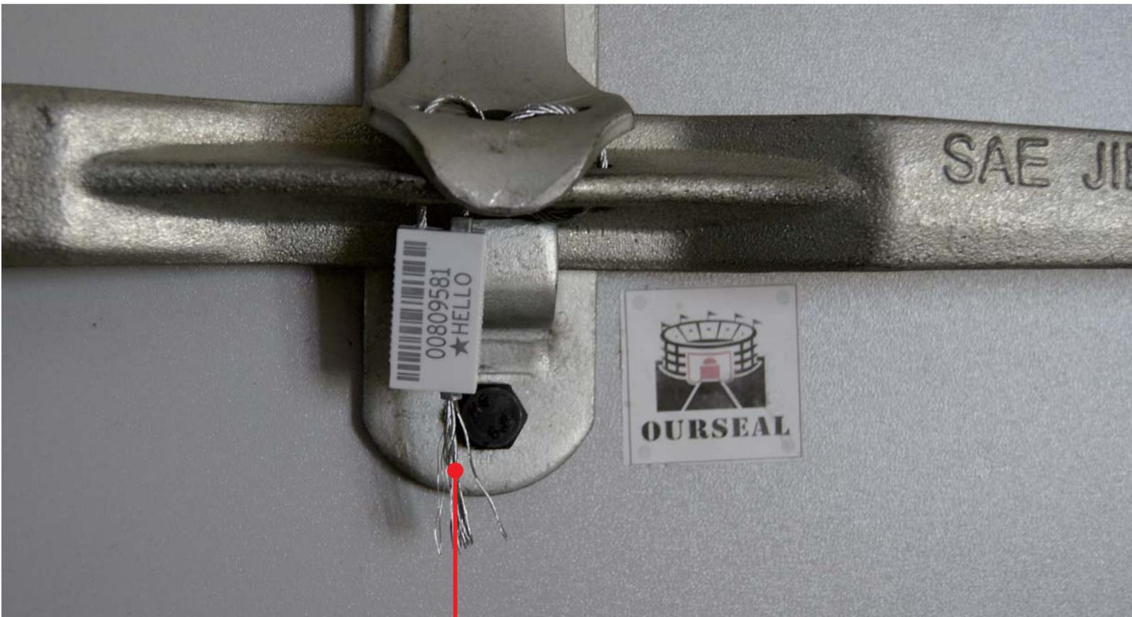
After seal, the wire end tip must be cutted.
